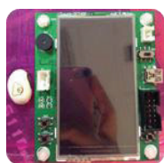
Fig. 1. EVB-TouchTFT400_v1.0 development board
